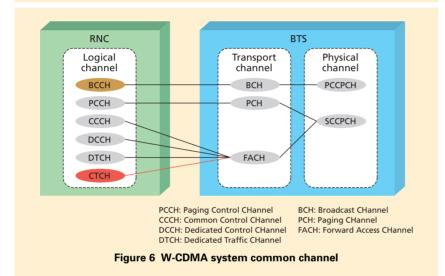
multiple transport channels<sup>\*11</sup> and logical channels<sup>\*12</sup> that the system requires are available on SCCPCH, and the CBS message is transmitted on one of them, the Common Traffic CHannel (CTCH) logical channel.
