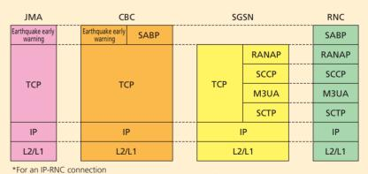
M3UA: Message transfer part 3 (MTP3) – User Adaptation layer SCTP: Stream Control Transmission Protocol
