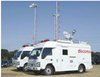
Satellite-entrance mobile base-station vehicles with satellite link
