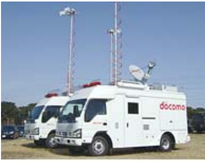
Mobile base-station vehicle equipped with satellite link
