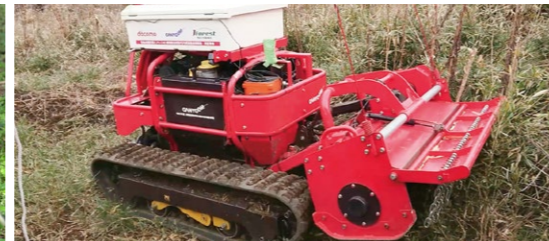
Remote control of a mowing machine using a DOCOMO network system
