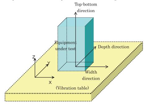
Figure 1 Simultaneous Excitation in 3 Directions (3-D Vibration Table)
