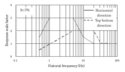
Figure 2 Acceleration Response Scale Factor of Excitation Waves (h = 3%)
