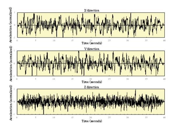
Figure 3 Time-based Excitation Waveforms (Maximum Acceleration normalized to 1)
