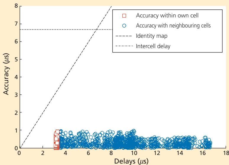
**Figure 8 Network synchronization accuracy with compensation of propagation delays**
