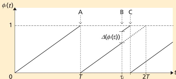
**Figure 1** Phase function of a pulse-coupled oscillator
