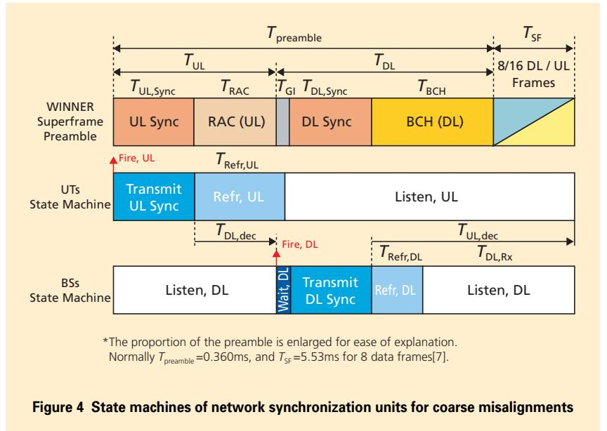
Figure 4 State machines of network synchronization units for coarse misalignments
