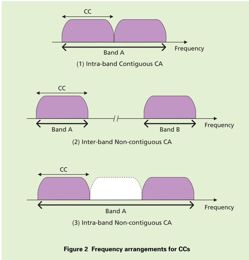
and the 800-MHz band. The use of two carriers can improve throughput in communications, and the use of multiple carriers with different propagation environments can improve stability.
