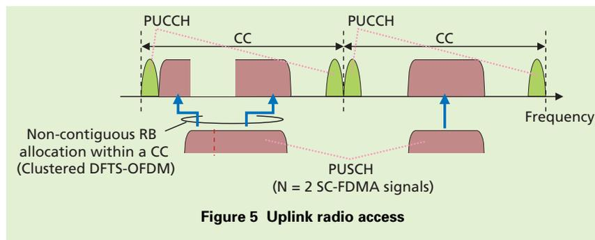
**Figure 5 Uplink radio access**
