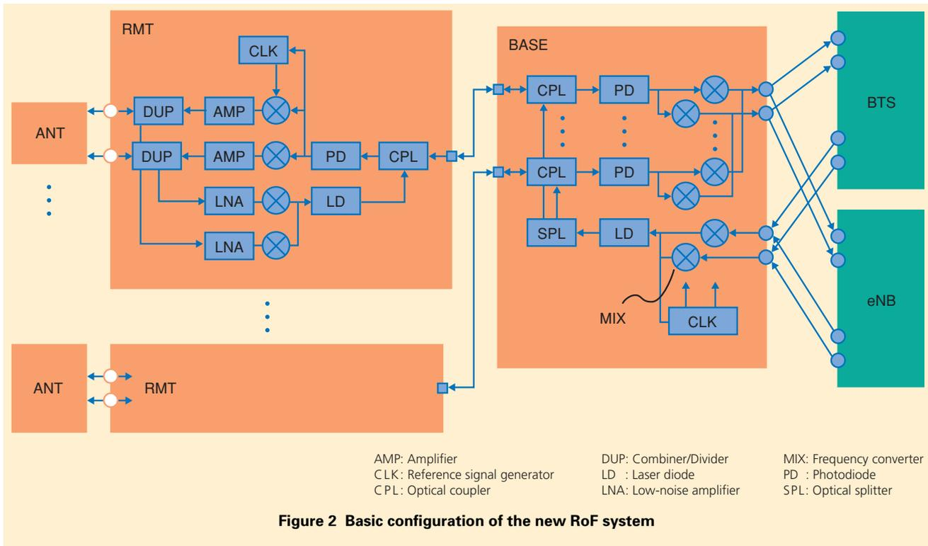
Figure 2 Basic configuration of the new RoF system
