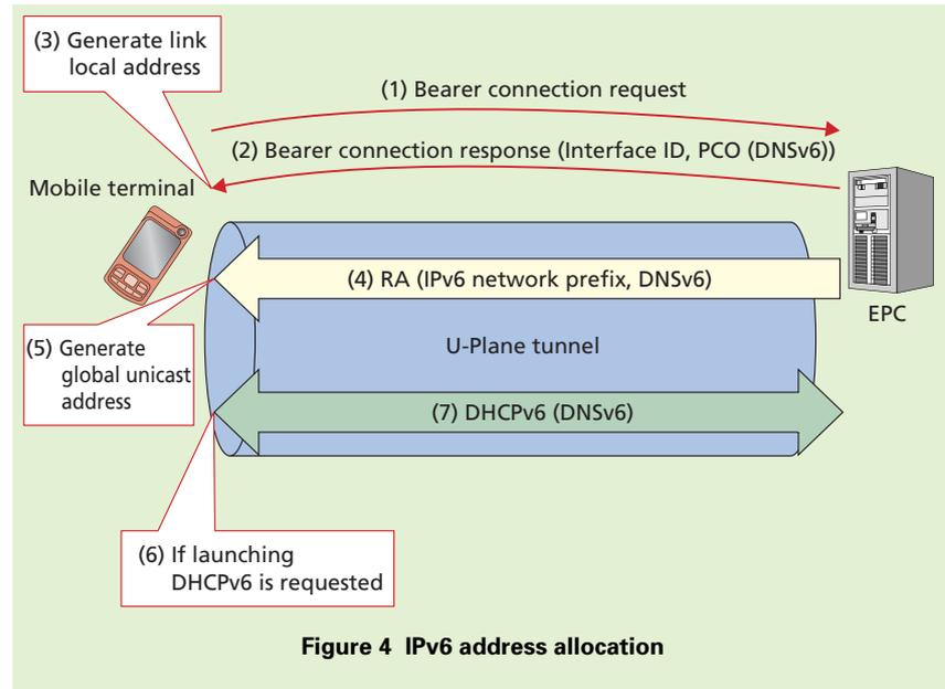
Figure 4 IPv6 address allocation
