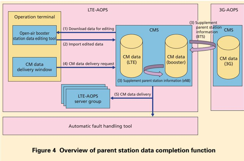
**Figure 4 Overview of parent station data completion function**
