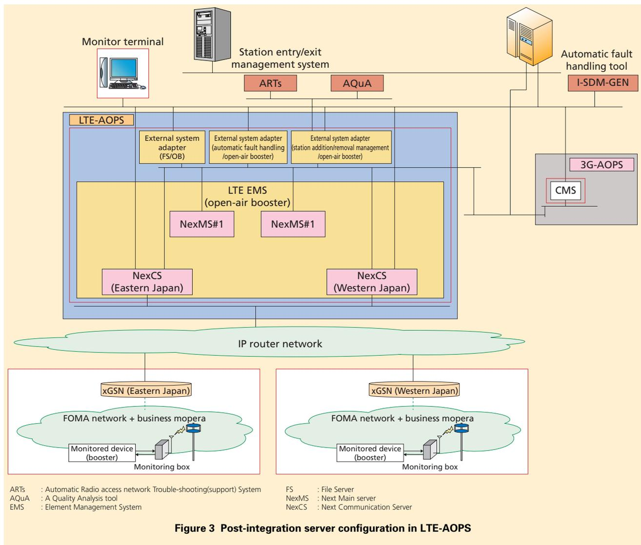
tional part that manages the configuration information of the 3G base station (Base Transport Station (BTS)) accommodated in 3G-AOPS.
