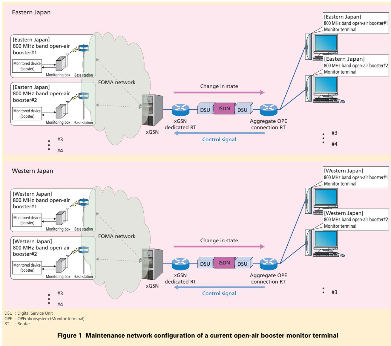
\*6 **xGSN**: A packet communication processing device in the FOMA network. It has both the Serving General packet radio service Support Node (SGSN) function and the Gateway General packet radio service Support Node (GGSN) function specified by 3GPP.
