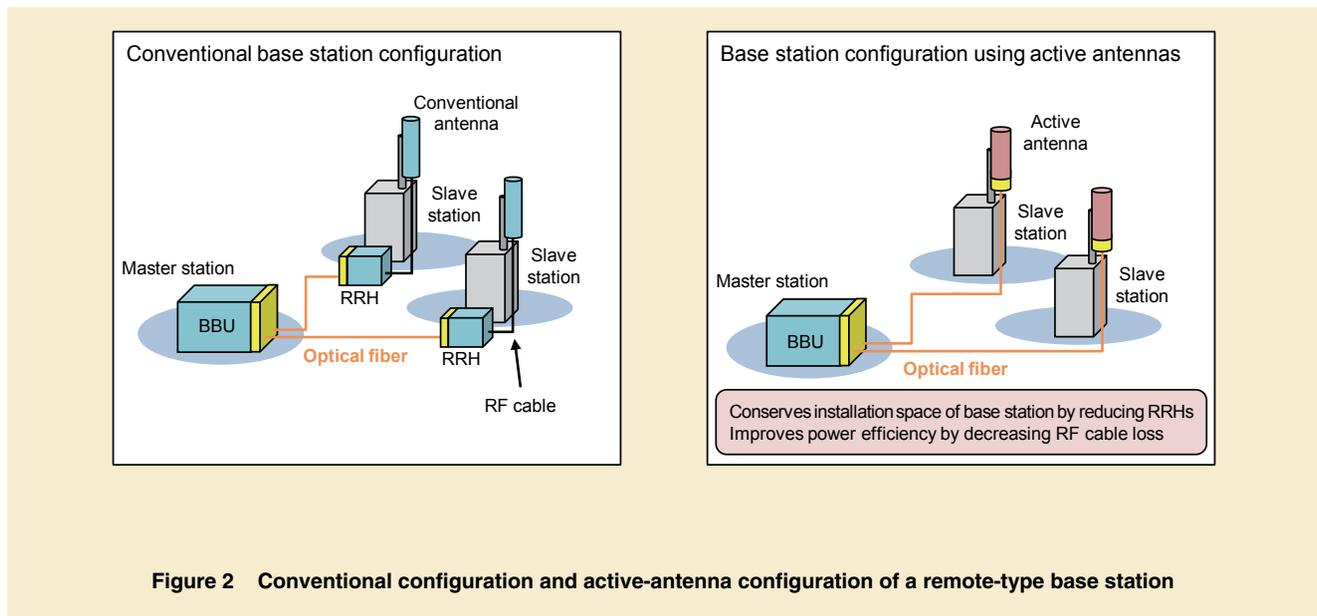
**Figure 2** Conventional configuration and active-antenna configuration of a remote-type base station
