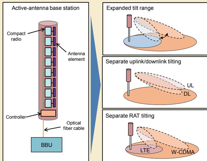
Figure 1 Configuration and features of active-antenna base station
