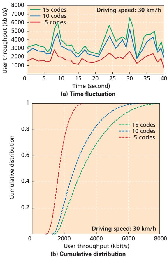
Figure 7 HSDPA throughput (field experiment, course A)
