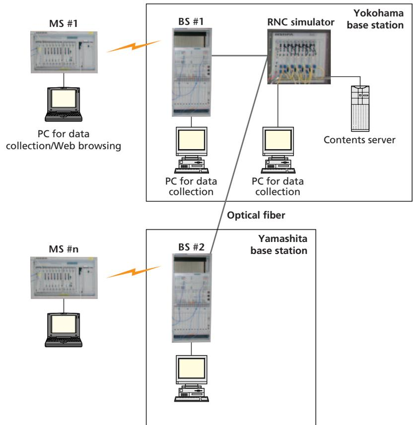
Figure 2 Experimental HSDPA transmission system
