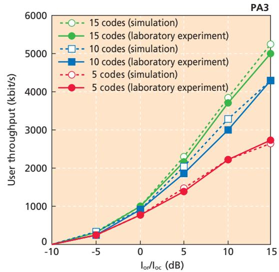
**Figure 4 HSDPA throughput (laboratory experiment)**
