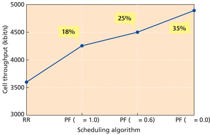
Figure 10 Cell throughput by scheduling algorithm
