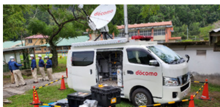
A mobile base station vehicle supporting an area affected by Typhoon No. 10 in 2020 (Kagoshima)
