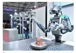
The remote-controlled robot, using "real haptics" technology and 5G, which enable tactile sensation information to be transmitted in real time, was displayed in the event. The feel of clay is fed back to the operator through the robot. The strengths of 5G, which include "low latency," provide a stable telecommunication speed and have helped create many different machines.
